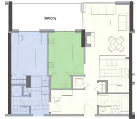
A "Lock-off" suite (image courtesy of SFU UniverCity) is a form of additional dwelling unit in multi-family buildings that acts as a secondary suite. The unit is sold as a two bedroom unit where the blue shaded unit can act as a 2 nd bedroom or as a separate one-bedroom suite that can be rented if not used or as a mortgage helper. The lock-off suite has its own entrance to the main corridor or from the main suite.
