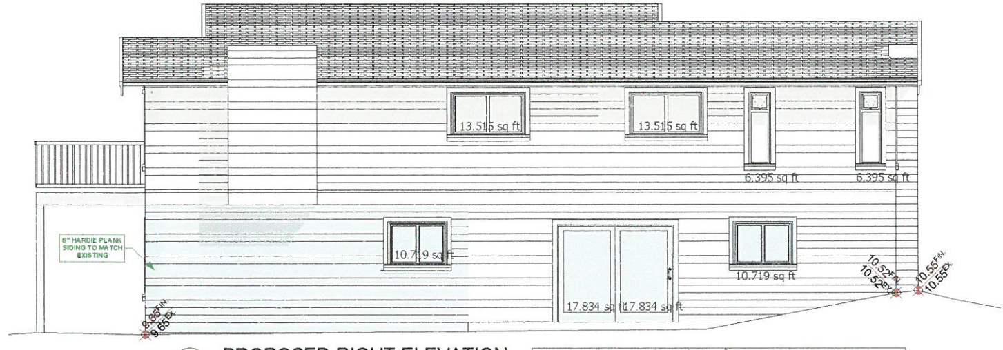
PROPOSED RIGHT ELEVATION SCALE: 1/4" = 1' - 0" EXPOSING BUILDING FACE: 81.01m 2 LIMITING DISTANCE: 3.03m AREA OF GLAZED OPENINGS: 7.15m 2 % GLAZED OPENINGS: 8.83% 45 min FIRE-RESISTANCE RATING: not required TYPE OF CLADDING: no limits PERMITTED % OF GLAZED OPENINGS (as per Table 9.10.15.4): 13.50% PERMITTED AGGREGATE AREA OF GLAZED OPENINGS: 10.94m 2
