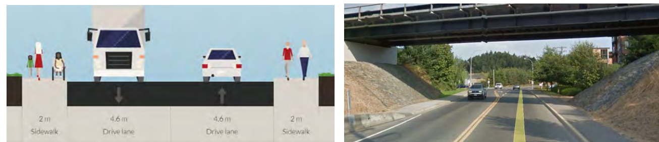
Figure 5.1: Existing Cross Section at Rail Bridge
