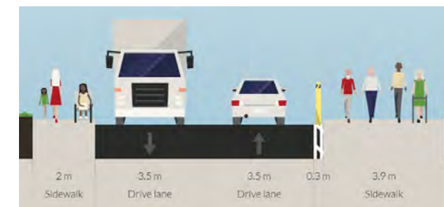
Figure 5.2: Preferred Cross Section Option
