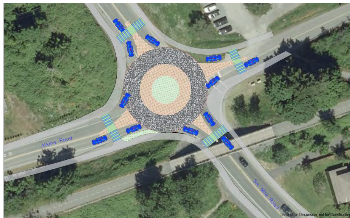
Figure 5.3: Conceptual Design of Atkins Road & Six Mile Road Intersection
